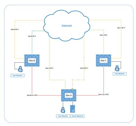
WAN Certification testing was developed to simulate a data center with two remote branches. The testbed therefore typically requires a minimum of three SD-WAN edge devices.
