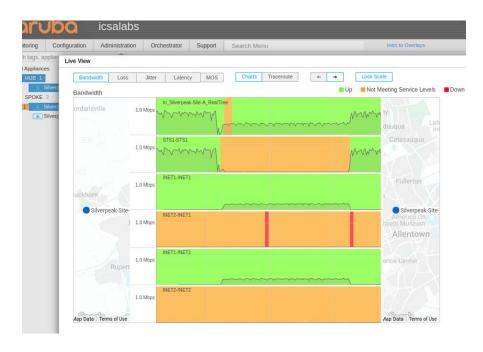
Fig. 4 – Traffic "Waterfalls" from one WAN path to another after degradation
