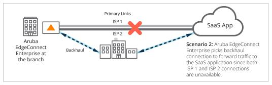
Figure 12: If both ISP 1 and ISP 2 connections become unavailable, EdgeConnect Enterprise automatically moves application traffic to the transport service configured as a backup that backhauls traffic through the data center.
