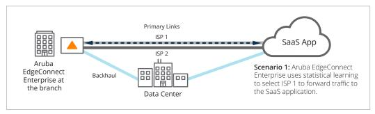
Figure 11: To optimize utilization of the provisioned WAN internet links (ISP 1 and ISP 2), Aruba EdgeConnect Enterprise monitors the performance of the two links by continuously measuring the packet loss, jitter, latency and mean opinion score (MOS) in real-time. In this example, based on statistical learning, Aruba EdgeConnect Enterprise dynamically selects ISP 1 to send traffic to the SaaS application since it is performing better than the ISP 2 service.
