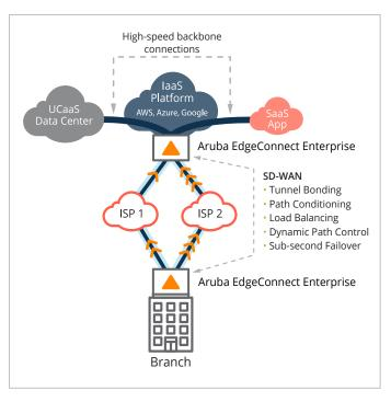
Figure 7: Aruba EdgeConnect Enterprise SD-WAN appliances deployed branch locations and in public clouds improve the performance and reliability of traffic across the "first mile" between the branch and the laaS platform. High-speed backbone connections in the cloud improve network quality and performance over the "last mile" between the laaS platform and SaaS infrastructure.
